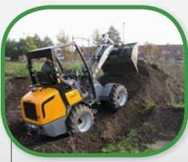
The GIANT V362 is with its 36 hp Kubota engine, the lightest loader in this range. This loader has regular axles (no planetary), one gear and speed up to 18 km/h. Because the motor cover can topple over, the new models are even better accessible for maintenance and service. These models are very suitable if you work on a flat surface and have to transport a load within a small area. These
